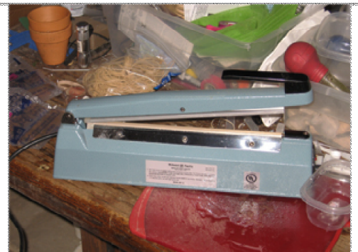
This is the Impulse sealer that seals the fish into channels in the breather bags.
